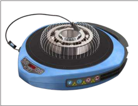
Fig. 1 – Magnetic field around bearing
